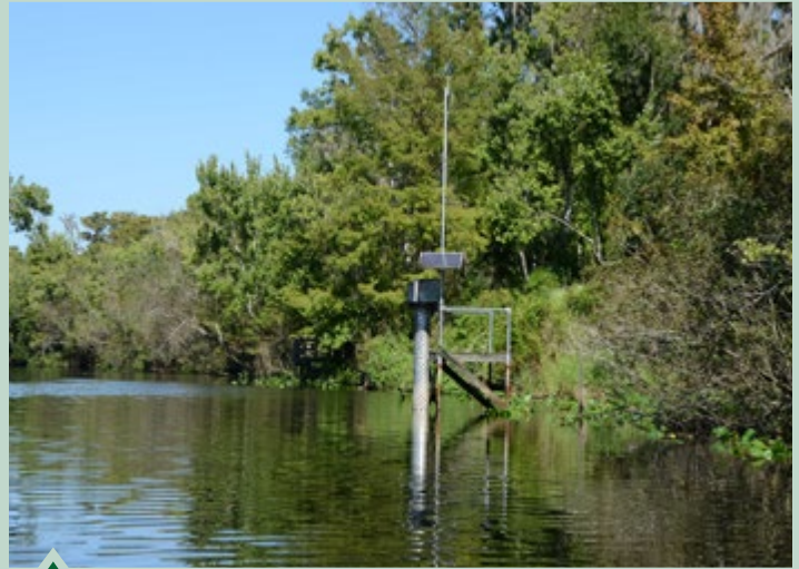
Hydrologic Monitoring Station on the Wekiva River
